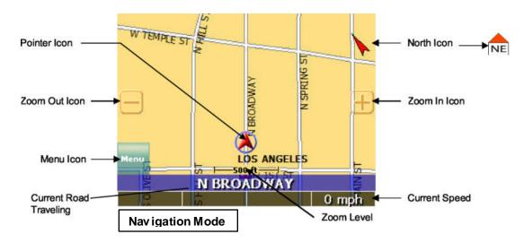
The pointer icon also indicates the signal strength of the satellite signals: Silver = no signal; **Red** = poor signal; **Yellow** = weak signal and **Green** = good signal.
